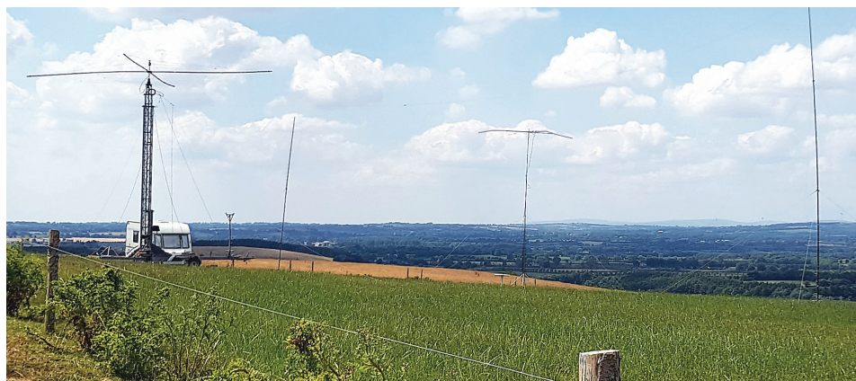
Olivier, ON4EI, won 1st-place worldwide in the Single Operator, Low Power, Phone category using this portable station from Ireland, operating as EI7T. His portable setup included (from left to right) the 15-meter-high antenna mast trailer not yet fully erected, with the Spiderbeam on top and the inverted V for 160/80/40 meters, a 1/4-wave vertical with 16 radials, the TA-33-JR Mosley antenna at 12 meters high, and an inverted L for 160/80 meters with 24 20-meter-long radials. [Olivier Vandenbalck, ON4EI, photo]
